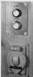
Figure 130B Start and Stop Buttons and Electrical Receptacle at Left Side of Machine
